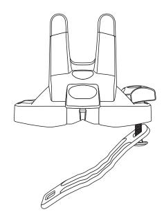
Position the base on the crossbar. Loosely install a bolt and knob as shown.
