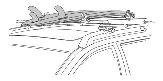
Adjust the position of the bases so that the bottom of the surfboard rests on the rubber part of the bases.
