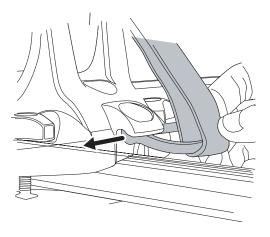
7. Rotate the buckle up to lock it to the base. Attach the buckle at the other end of the strap to the other base and lock it in place.
